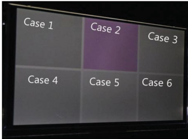
Figure 6. The picture of 7" split test 3D display samples for color moire test taken in oblique direction.
